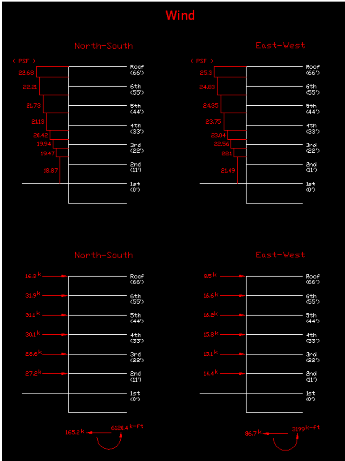
Figure 10 – Wind Pressures and Story Forces
